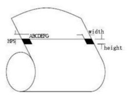
Printed lacation:is shown as chart above, the black mark should be printed to character surface of right or left side rim.
