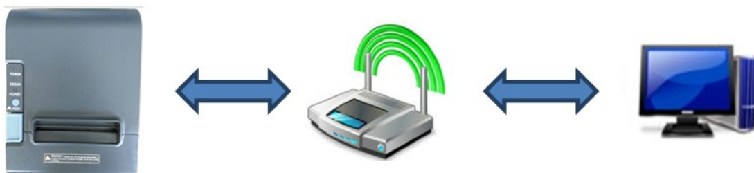
Exemplo 2: IP TP-450 192.168.0.180...IP Roteador 192.168.0.1.....IP Computador 192.168.0.150
