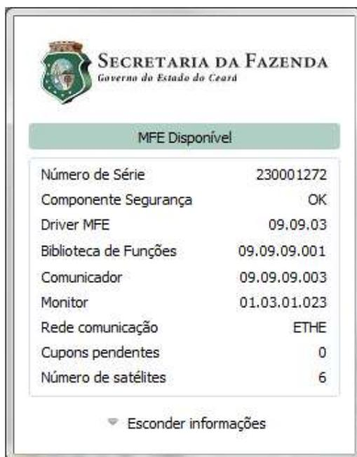
**Figura 17 - Monitor do Driver MFE – tela de status expandida**
